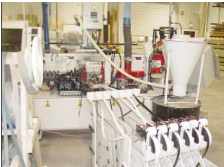
A seven-spool edgebanding material cart aids in switching from one edging to another to streamline the edgebanding process.
